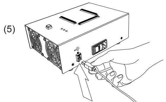
5. Directly connect USB cable to type B USB port on programmer.
